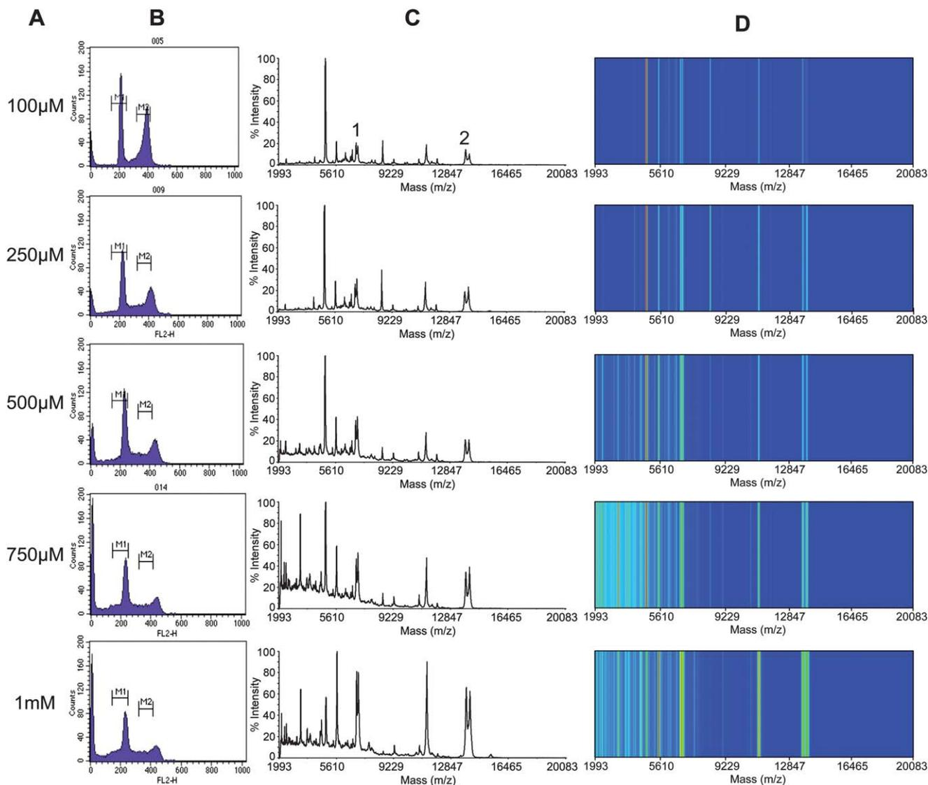
**Fig. 5** Comparison of flow cytometry and intact cell MALDI TOF MS in dead cell detection. (A) Concentrations of pro-apoptotic compound andrographolide used to treat HeLa cells. (B) Propidium iodide-labeled DNA profiles of the treated cells as measured by flow cytometry. (C) Intact cell MALDI TOF MS of the same samples. (D) MALDI mass spectra presented in barcode view.
