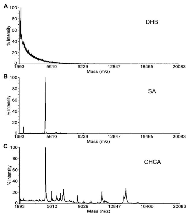
**Fig. 1** MALDI mass spectra of HeLa cells with different matrix solutions. (A) 10 mg DHB per mL ACN/0.1% TFA (7/3, v/v), (B) 10 mg SA per mL ACN/0.1% TFA (7/3, v/v), and (C) 10 mg CHCA per mL ACN/0.1% TFA (7/3, v/v).
