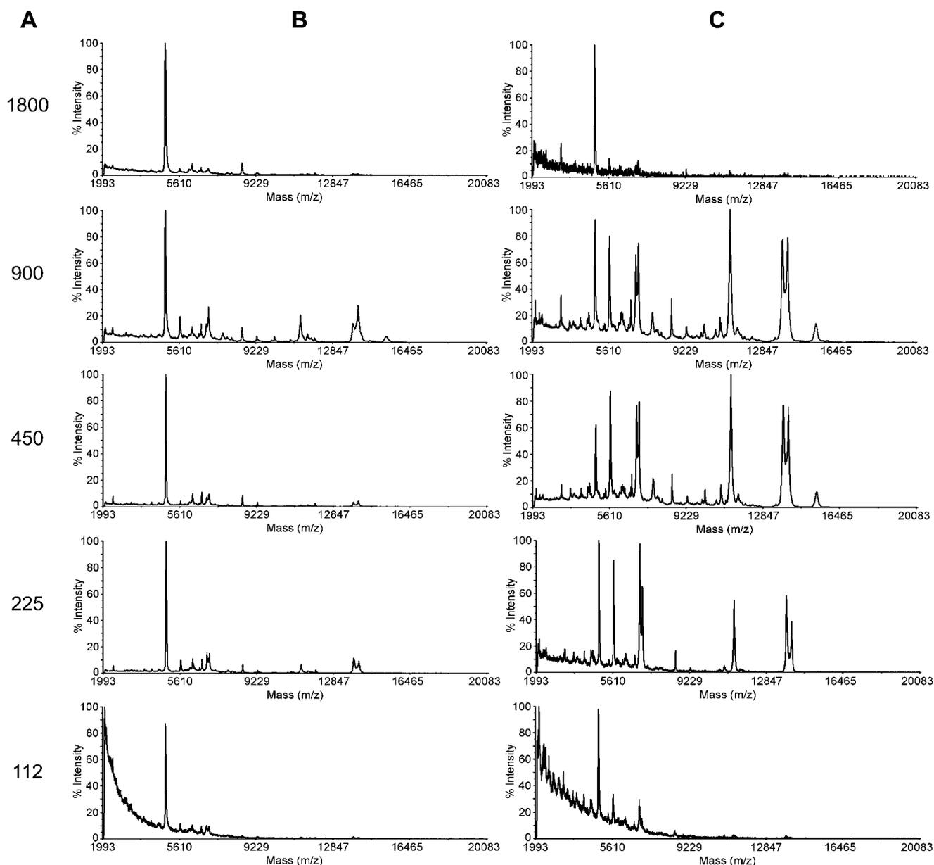
**Fig. 2** Comparison of MALDI mass fingerprints of HeLa cells at different cell numbers per spot on the MALDI target. (A) Cell numbers on each spot, (B) MALDI TOF mass spectra of viable cells, and (C) MALDI TOF mass spectra of apoptotic cells.
