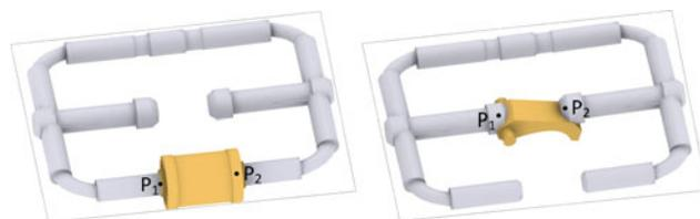
Fig. 6. Illustration of Eq (1). A new element (yellow) is placed into a proxy (black lines), intersecting with existing elements at  $P_i$ . Left: we prefer to place the element forming two good connections with existing elements near the boundary of the proxy. Right: we prefer to place the element forming two bad connections near the proxy center.
