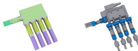
Fig. 14. A hand proxy (left), with manually specified joints in blue (right). Other elements are automatically filled.
