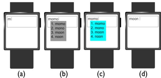
**Figure 4:** A storyboard illustrating a user entering "moon" with *FingerT9*. (a) Type by tapping a key on finger segment. (b) Type the word letter by letter. Candidate list is displayed. (c) The user taps the "select" key. Candidate list turns to cyan to indicate selection is triggered. (d) The user taps "3" to confirm selection of third candidate.
